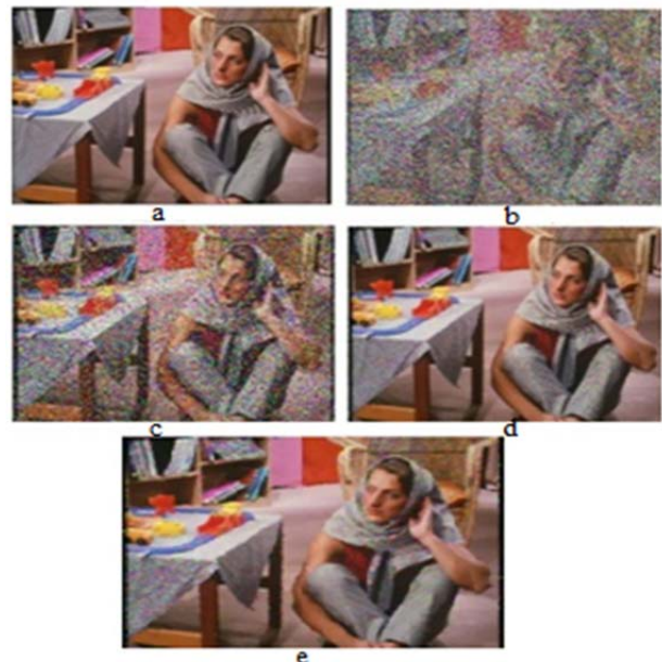
Figure 10: a) Input Image b) 60% Noisy Image c) Median Filtered Image d) SSMF Result e) MSP result
